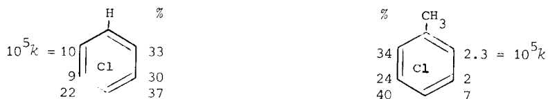
Fig. 1 Orientation and associated rate constants for fluorodechlorination of pentachlorobenzene ( 250^\circ ) and pentachlorotoluene ( 275^\circ )
